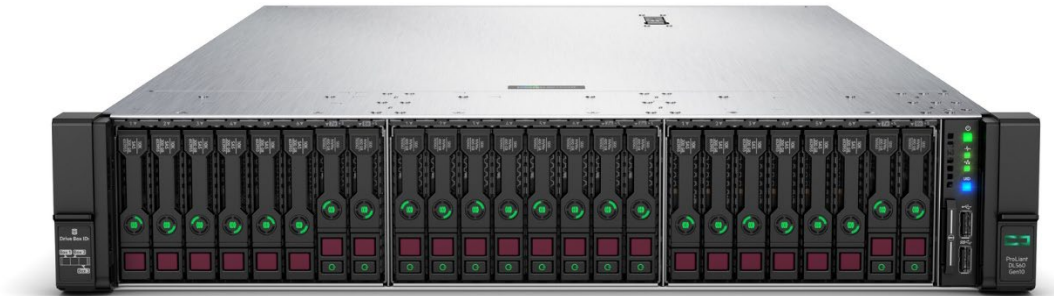
24 SFF (incl 12 NVMe SSDs) hot-plug drive model
